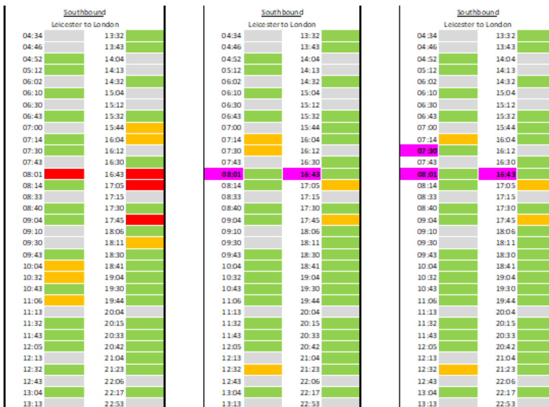
21.2 Figure 21 shows that the capacity issues experienced in the base scenario are resolved with the introduction of the Class 810 rolling stock however it should be noted that it has been assumed that ten car units would be used on six of the services departing London and three of the services departing Leicester in the 2030 growth scenario, these are indicated by the highlighted departure time text.
