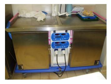
The trolley is completely portable as it is fitted with wheels. The trolley is used to reheat frozen multi portion meals and to cook fresh food from scratch. This has been identified
